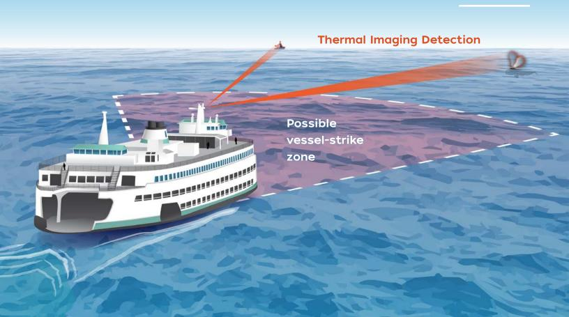
on ships, the systems can automatically alert shipping captains to the presence of whales up to several kilometers away within seconds, enough time for most vessels to slow down or change course.
